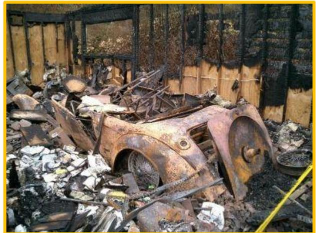
1937 T57 Bugatti. The owner flooded the engine while starting the car, the gas pooling on the floor. It backfired, starting the fire. The elderly man was unable to get the fire extinguisher to work.
